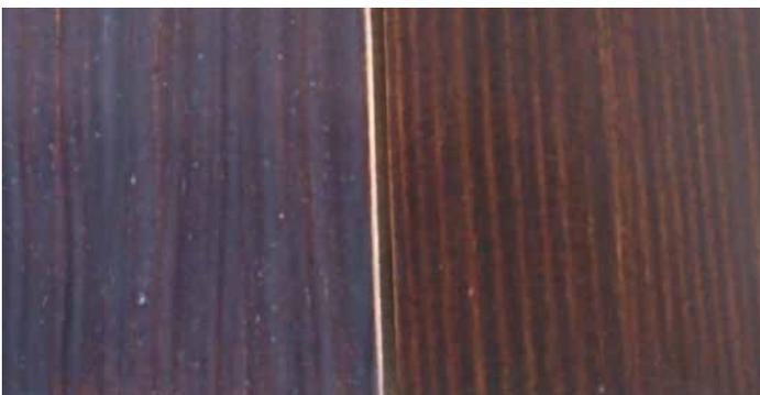
If the dispersion of particles in the coating is not achieved (left picture of a board), the particles agglomerate and the coating becomes non-transparent and its light absorption quality diminishes. Once the conditions for a good dispersion of particles (homogeneous coating) and coating stability are met, the coating containing the CCR is transparent (right picture of a board) and has good absorption qualities.
