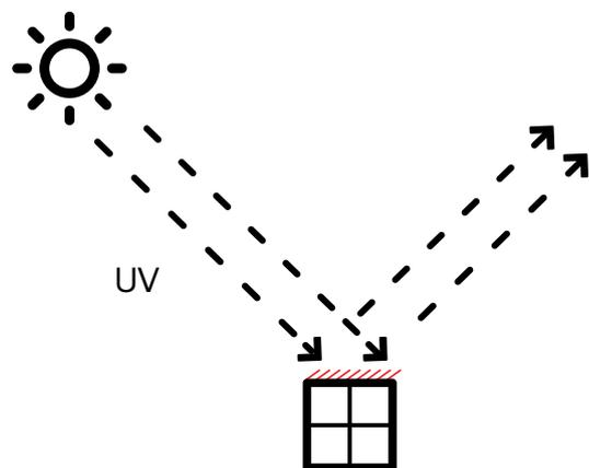
Protective coating with nano  $\text{TiO}_2$
