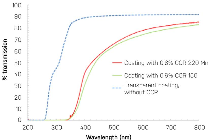
The effect of CCR addition into the coating. The addition of CCR improves the level of UV absorption in comparison with the basic coating without a UV absorber. By increasing the CCR content, the UV light absorption level is additionally increased.
